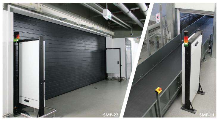
**SMP-11** or **SMP-22** Radiation Portal Monitors (RPMs) are equipped with one or two measuring columns, respectively, to perform functions of detection and preliminary processing of the signals, and a control panel with a touch screen and printer.
