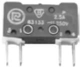
83 133      | Basic miniature switch with a double-break change-over contact of the same polarity, with four terminals running in parallel to the longitudinal axis of the drive element, and with sleeves in assembly holes - with the L1 soldered terminals, and with gold-flashed terminals             | 59-691022     | 2.1        |
